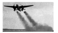
Douglas A-20A Havoc takes off using liquidpropellant rocket JATO from Muroc (now Edwards AFB) [Courtesy JPL 383-93 1942].
